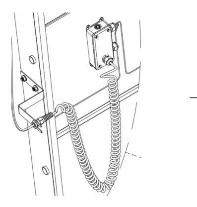
1. A torsion-resistant waterproof connector is installed on the spring wire bracket, and then fixed on the side of the door frame by bolts, and the long straight end of the spring wire passes through the torsion-resistant waterproof connector to connect to the motor.
