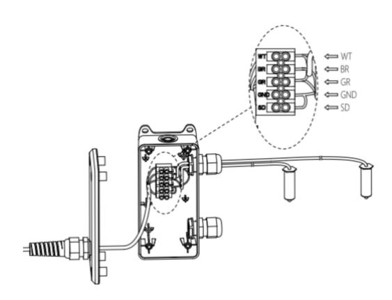
1. The spring wire is connected to the left side of the wiring terminal in the safety junction box, and WT and GND need to be short-circuited.
