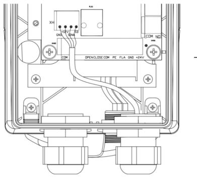
1. To connect the spring wire to the motor, you need to remove the 8.2K resistor and short wire from the original safety terminal, and then connect the spring wire to the safety terminal from left to right according to the color of the wire.
